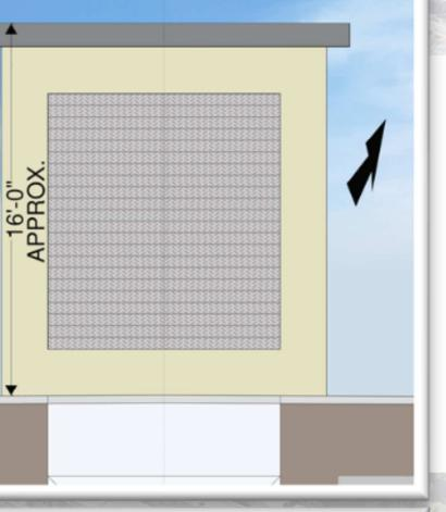
**Air Ventilation Structures 5** locations located between Eastbound and Westbound tunnels spaced at approx. 600'
